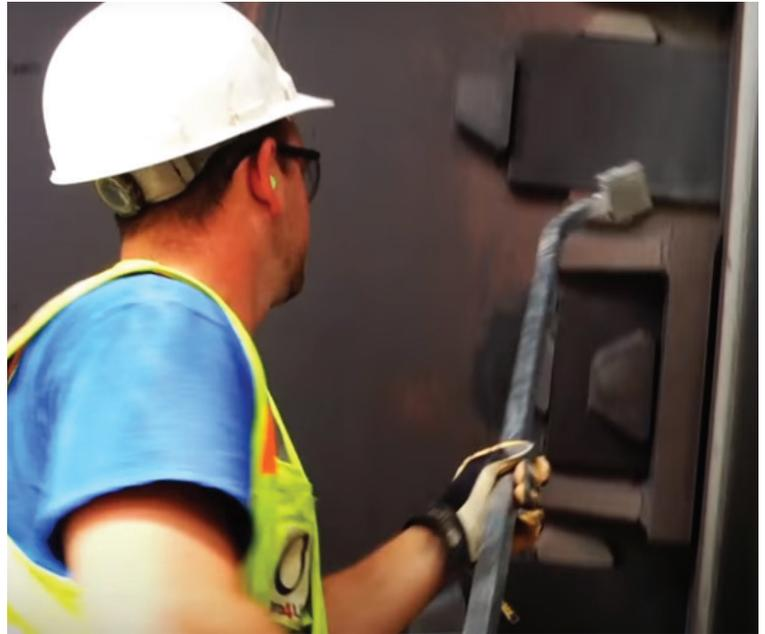
*Our lightweight, 5-foot-long Easy Bar® Lubricator insertion tool has a flexible neck that can be easily angled for swift application. The tool is specially designed to firmly hold any Easy Bar without interfering with the release of the bar.*
